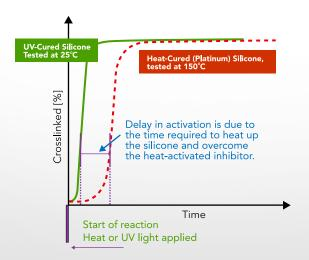
**ReliaSil UV HCR** optimizes the addition-cure reaction with the incorporation of a UV-sensitive inhibitor that replaces the standard heat- sensitive inhibitor.
