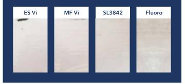
In testing, SilForce SL3842 release coating provided an almost 10X reduction in initiation spike and smoother release when delaminating the liner from bitumen mastic as compared to a typical vinyl end-stopped polymer.
