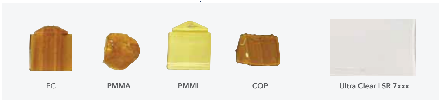
Figure 3: Thermal aging for 6,480 hours at 150 °C for observed yellowing on a variety of transparent materials, including the LSR 7xxx series
