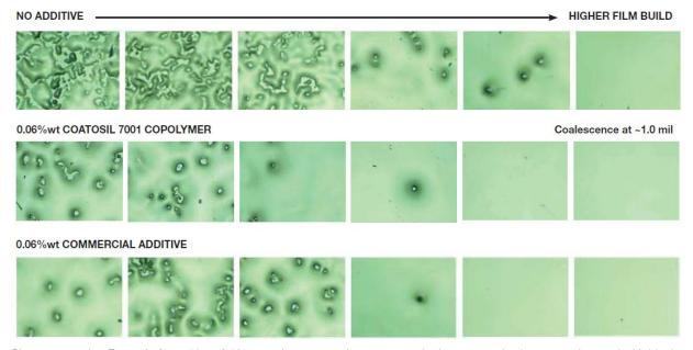
Clearcoat coating **Formulations #1 and #2** were also prepared over a smooth electrocoated substrate and coated with black basecoat. The Chrysler C-Box and Wave-Scan Dual results are shown for the following systems: No additive, 0.06%wt CoatOSil 7001 copolymer, and 0.06%wt of a Commercial control on a 100gram resin solids basis. Clearcoat film builds were in the ~2.0 to 2.3mil film thickness range for all topcoats.
