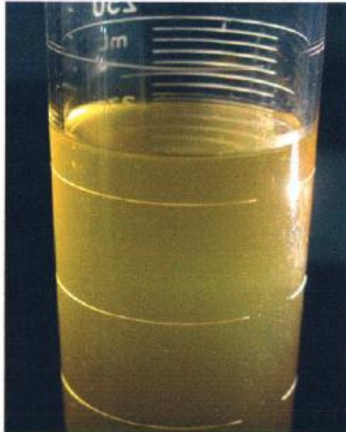
Figure 2: SAG 1572 silicone antifoam emulsion at 0.3% use level in a non-ionic spray adjuvant formulation.
