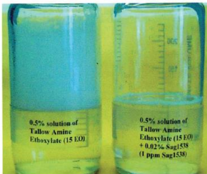
Figure 2: SAG 1538 Silicone Antifoam Defoaming in Tallow Amine Ethoxylate (0.5%)
