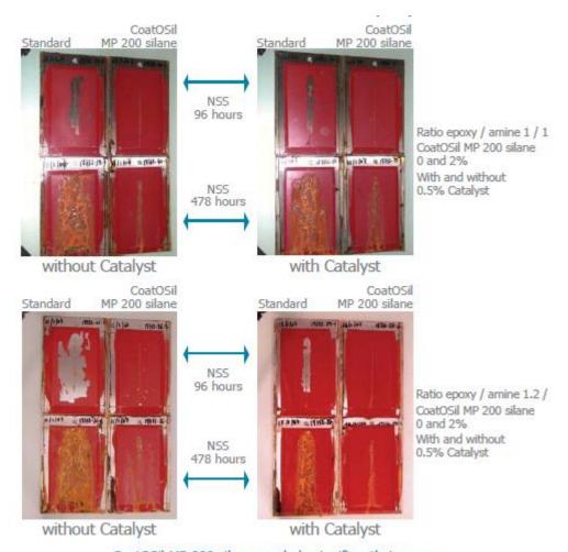
CoatOSil MP 200 silane can help significantly increase the corrosion resistance of 2K HS epoxy primer. It can lower the impact of epoxy/amine ratio and catalyst content.
