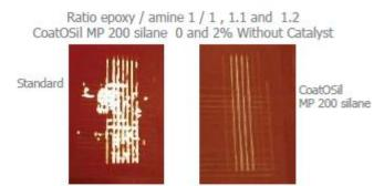
CoatOSil MP 200 silane can help significantly increase the adhesion performances of 2K HS epoxy primer.
