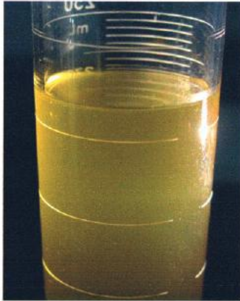
Figure 2: SAG 1572 silicone antifoam emulsion at 0.3% use level in a non-ionic spray adjuvant formulation.
