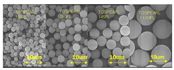
SEM illustrates the uniform size distribution of the spherical 2, 3, 4.5 and 10-micron beads.
